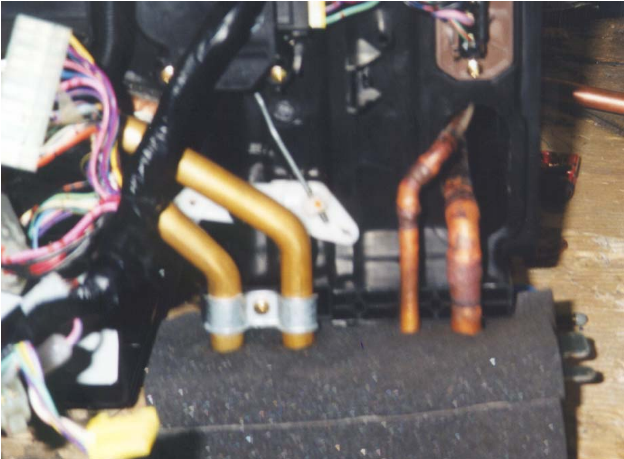
Side of evaporator housing assembly showing tubing routing out and down through seal material for floor.
